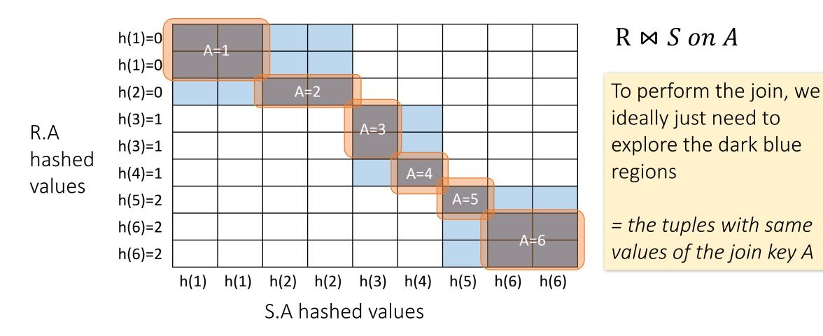
$R \bowtie S \text{ on } A$ h(1)=0 h(1)=0 With a join algorithm like h(2)=0 BNLJ that doesn't take h(3)=1 R.A advantage of equijoin h(3)=1 hashed structure, we'd have to h(4)=1 values explore this whole grid! h(5)=2 h(6)=2 h(6)=2 h(2) h(3) h(4) h(5) h(6) h(6) h(1) h(1) h(2) S.A hashed values
